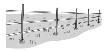
Plastic posts are placed along each edge of the enclosure from corner to corner.
